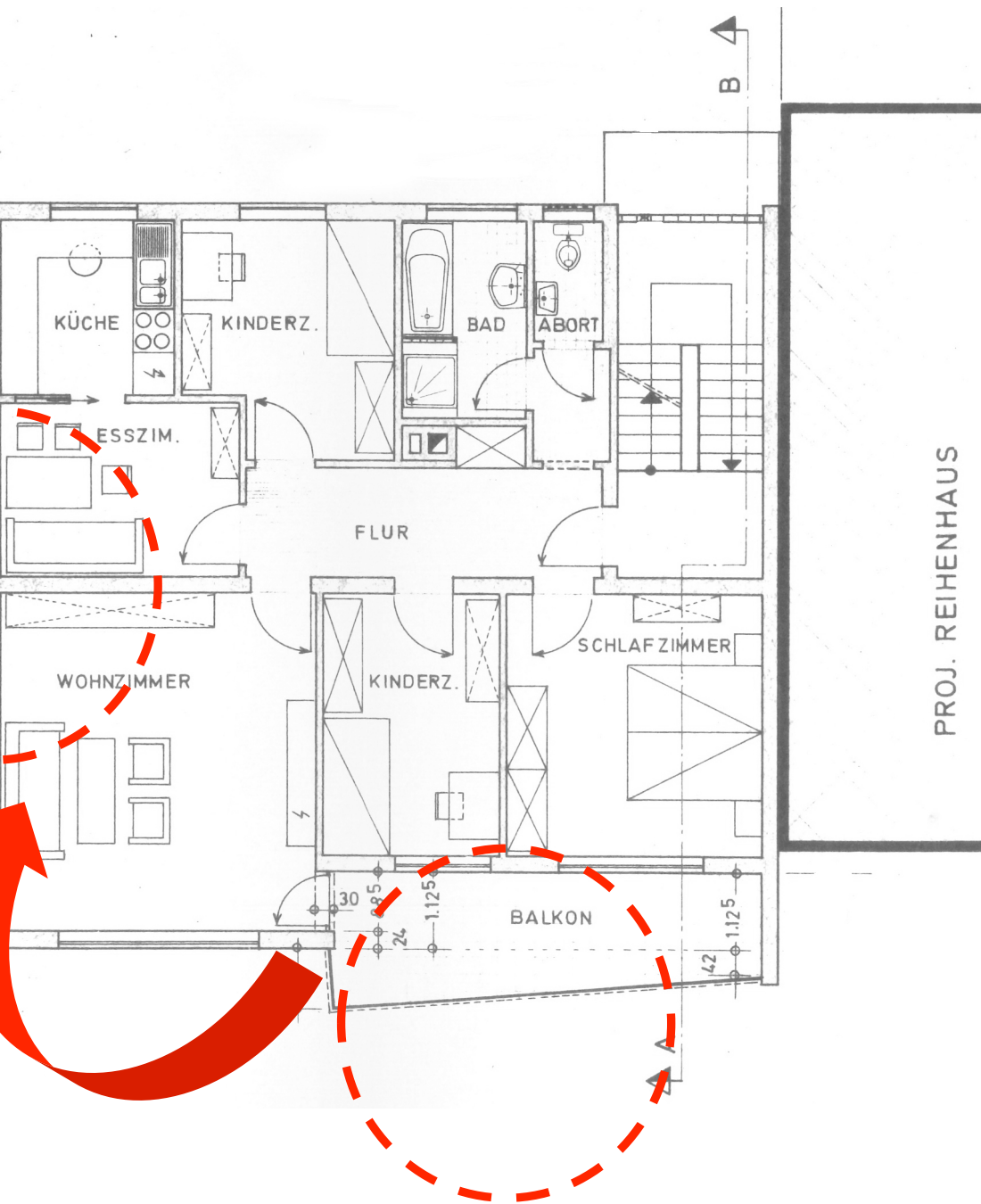
Demolition of the existing balcony on the south facade
